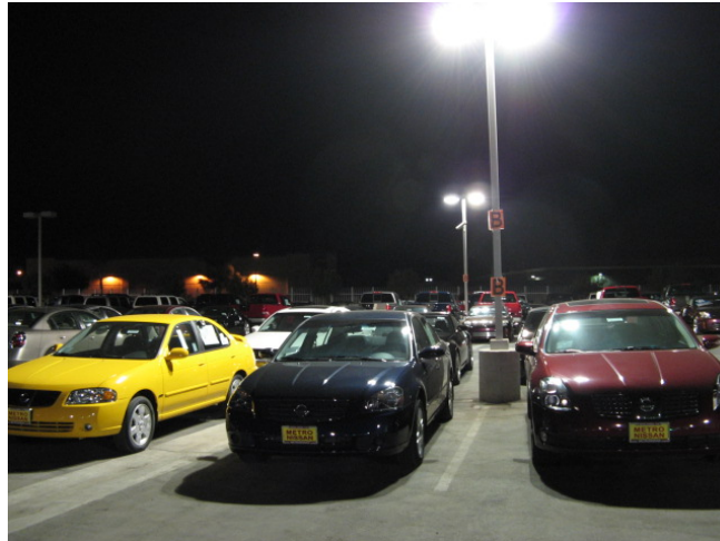
Figure 12: System B – 750 W Metal Halide – Night
